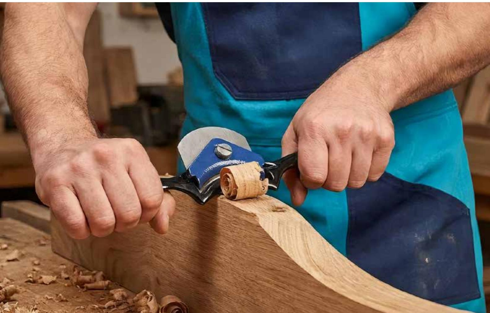
This tool combines strength, reliability, and ease of use for outstanding woodworking results. Its adjustable carbon steel blade ensures precise scraping and clean finishes, while the solid cast iron body adds long-lasting stability. Designed with ergonomically shaped handles, it offers comfortable grip and steady control during detailed work. Perfect for refining and preparing wooden surfaces, it helps achieve a smooth foundation ready for staining or varnishing.
