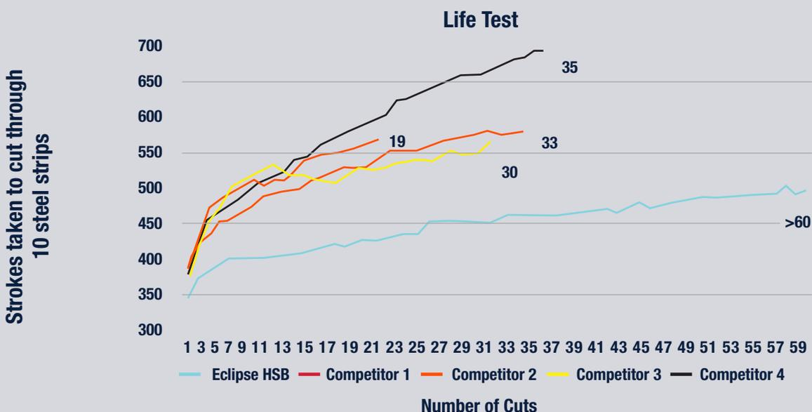
RESULT: Eclipse Bimetal blade is significantly quicker through the first cut than competitor blades.
