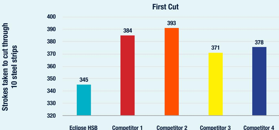
RESULT: Eclipse Bimetal blade is significantly quicker through the first cut than competitor blades.
